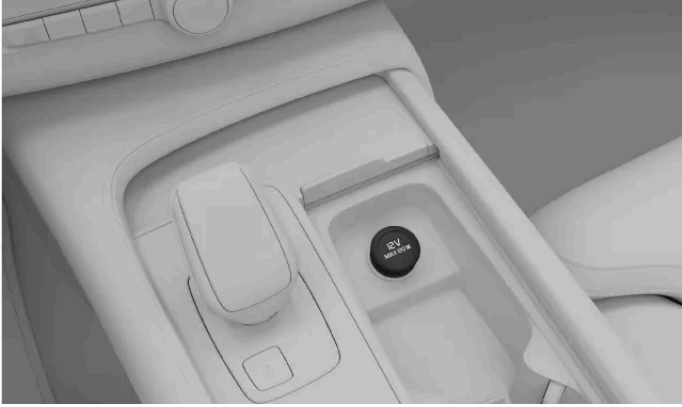
The 12 V socket in the center console
