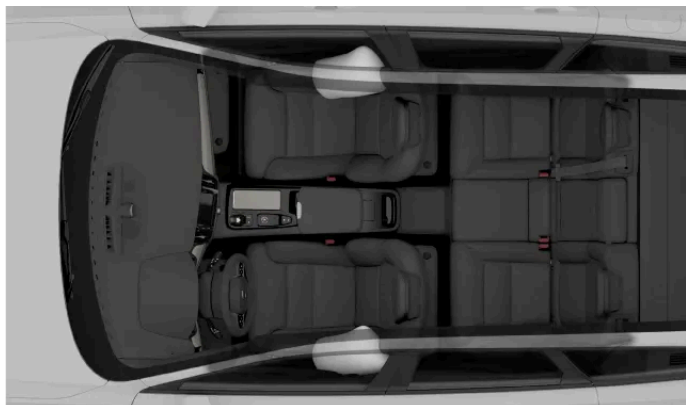
Side-collision airbags for the front occupants.
