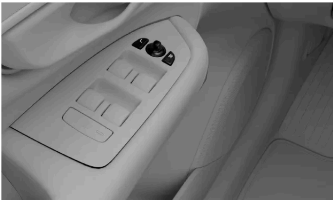
Controls for adjusting the door mirrors
