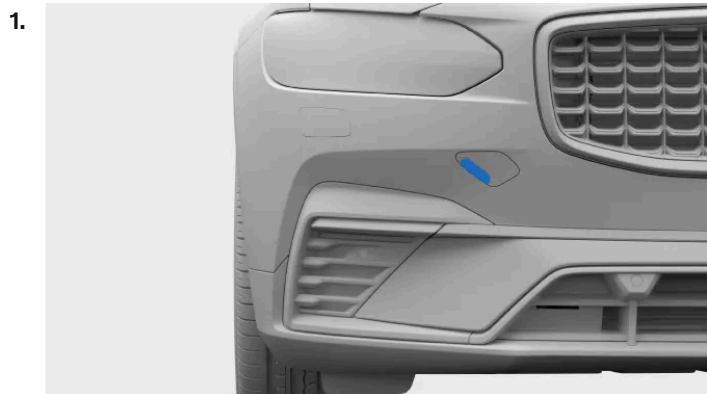
Front towing eye fastening cover
