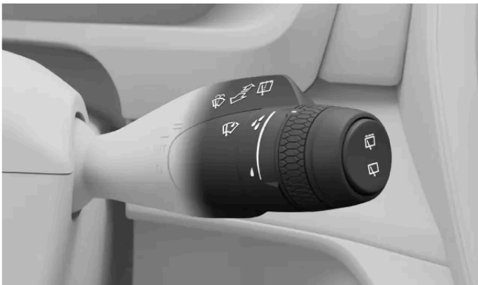
Right-hand steering wheel stalk
