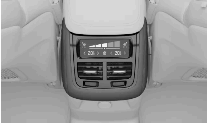
Climate controls in center console
