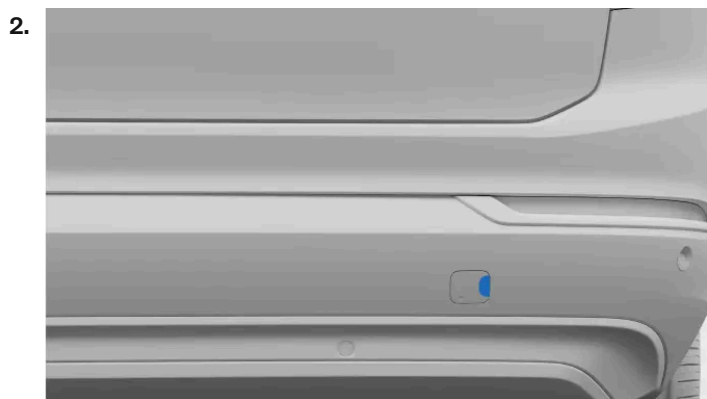
Rear towing eye fastening cover
