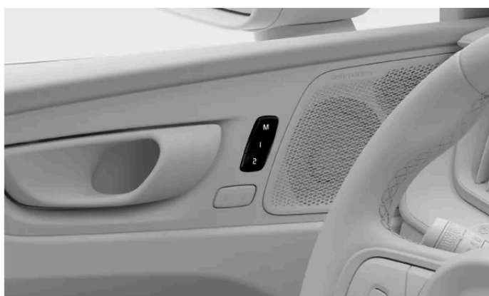
Location of the preset seat adjustment buttons
