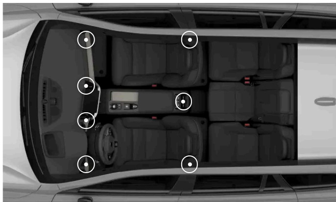
The locations of the adjustable air vents
