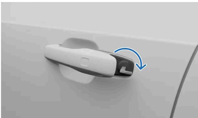
5. Turn the key back 45 degrees counter-clockwise back to its starting position and remove it.
