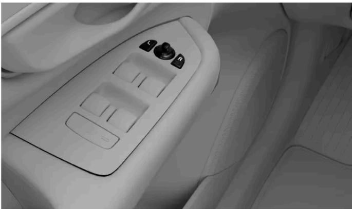
Controls for adjusting the door mirrors
