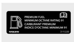
Premium fuel label is located on the inside of the fuel filler flap on vehicles that require premium fuel.
