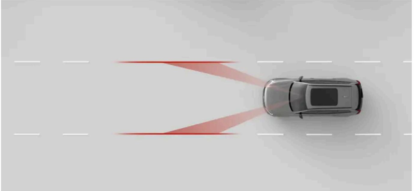
When lane keeping aid is enabled, the vehicle can alert you if you are about to drift out of your lane, and it can ask you to steer the vehicle with attention. It can also perform steering interventions. The lane keeping aid relies on the vehicle's forward-facing camera to identify road markings and your position in the lane.
