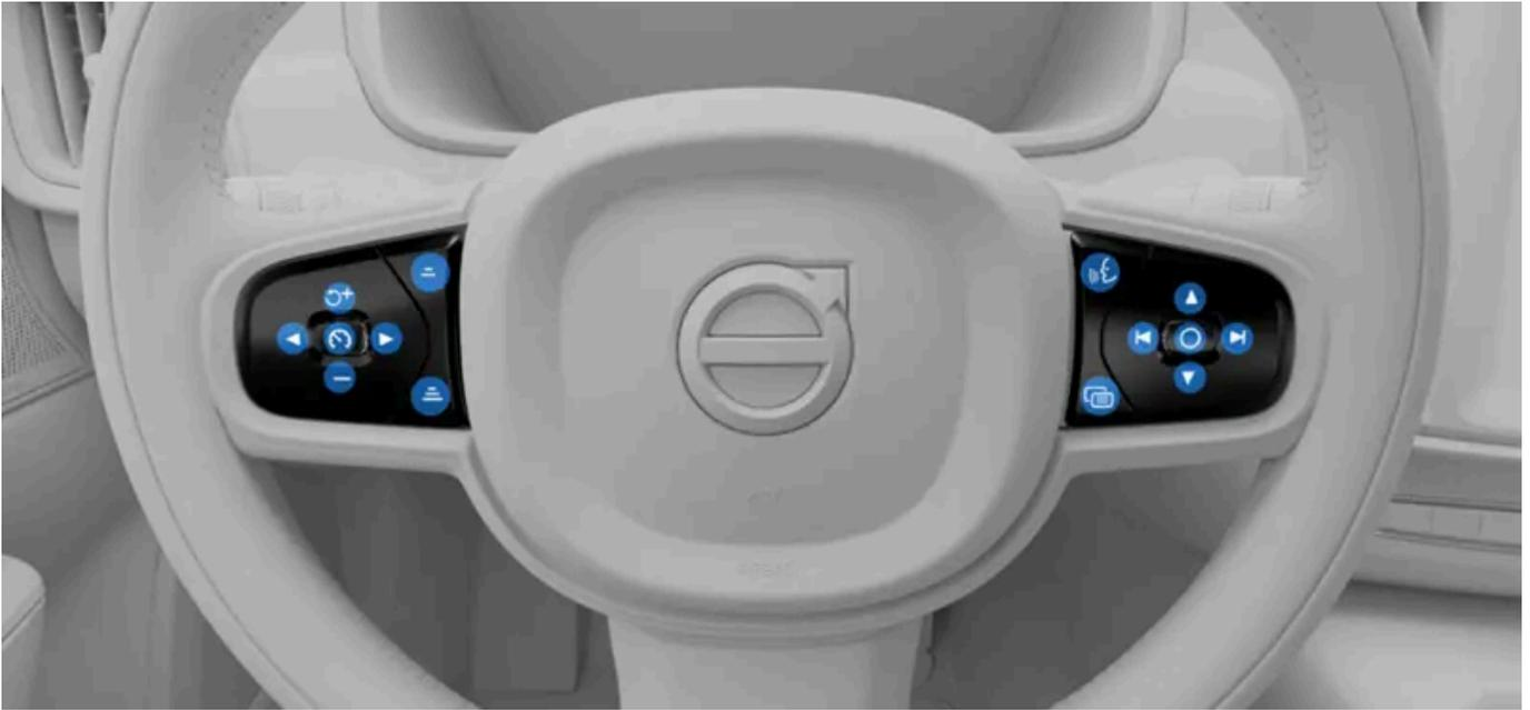
The buttons on your steering wheel's left-hand side control the driver support features.
