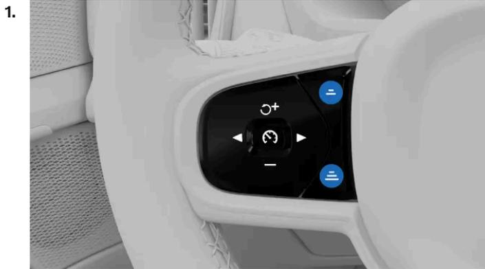
Adjust the time interval to vehicles ahead using the buttons on the steering wheel.
