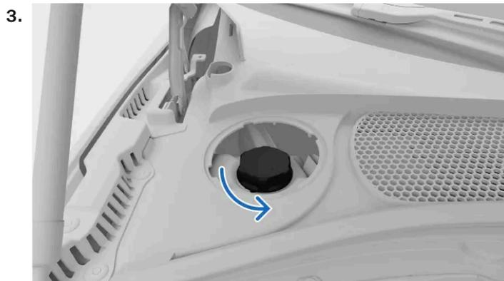
Unscrew the coolant reservoir cap.
