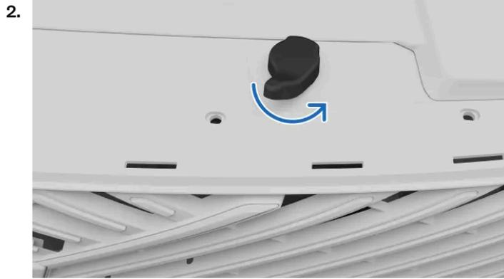
Locate the second lever below the front edge of the hood and rotate it counter-clockwise.
