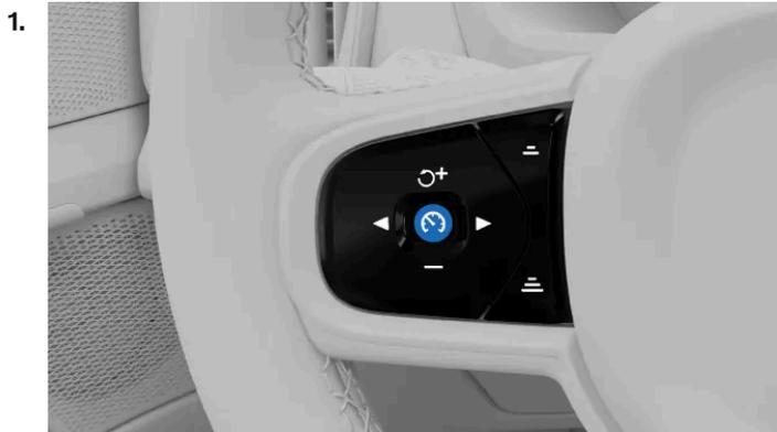
When it's safe to do so, press the Pilot Assist button
