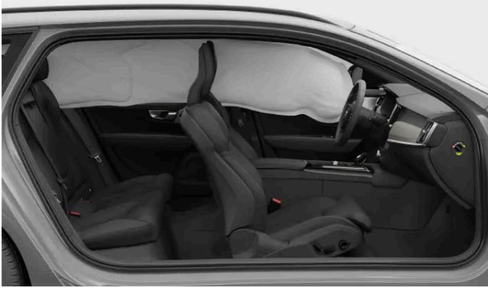
Inflatable curtain deployed on one side of the vehicle.
