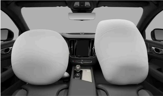
The driver side has two front airbags. The upper airbag is packed inside the steering wheel and the knee airbag is packed behind a panel below the steering wheel.
