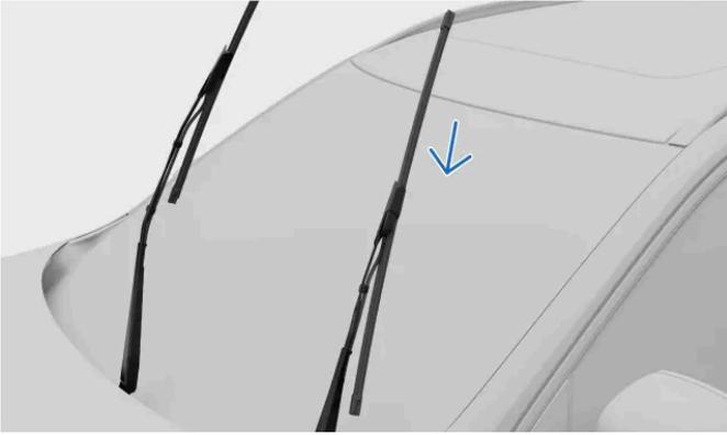
Make sure that the blade for the driver side is longer than the blade for the passenger side. Slide the wiper blade onto the wiper arm. Ensure that the pin on the wiper arm goes into the hole on the wiper blade. Push the blade into the wiper arm until you hear a click.
