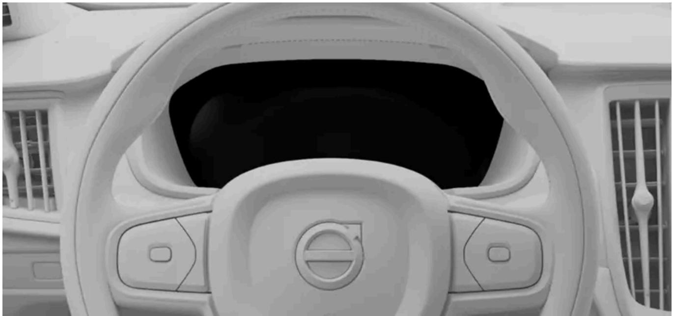
The instrument panel is located in front of the driver, behind the steering wheel.
