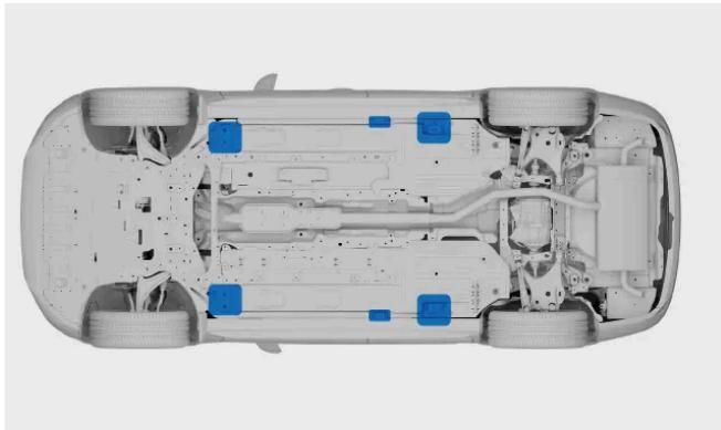
There are two jacking points on each side of the vehicle.
