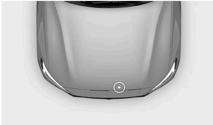
The second lever is below the front edge of the hood, on the driver's side.
