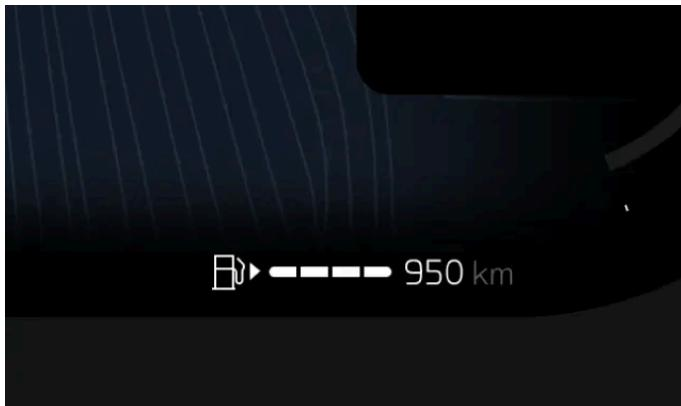
Your range is primarily related to the amount of fuel left in the tank and your driving practices, but external conditions can also be a factor. The fuel meter and expected range are displayed in the instrument panel.
