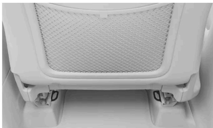
The lower tether attachment points can be found at the back of the floor rails of the front seats.
