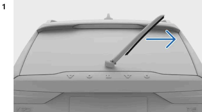
Grasp the center of the wiper arm and lift it up and away from the rear windshield. You may feel some resistance halfway – this is the lock position. You need to pull the wiper arm past the lock position so that it doesn't fall back onto the windshield
