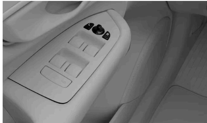
Controls for adjusting the door mirrors
