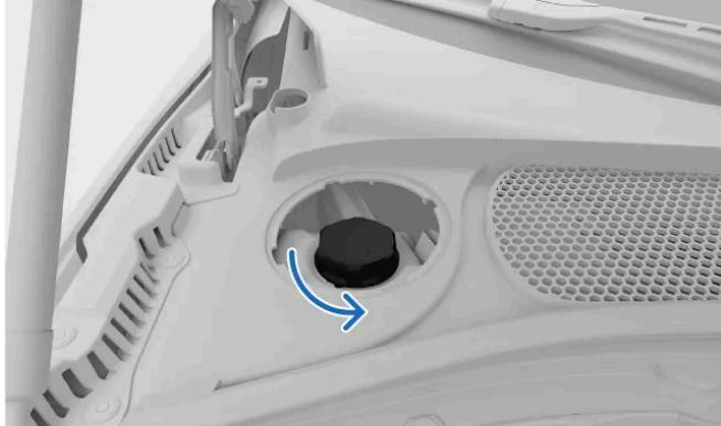
Unscrew the coolant reservoir cap.
