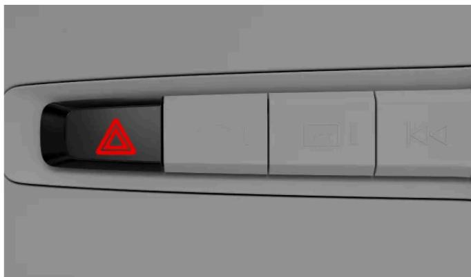
The location of the hazard warning lights button below the center display
