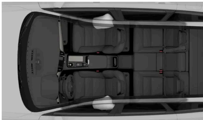
Side-collision airbags for the front occupants.
