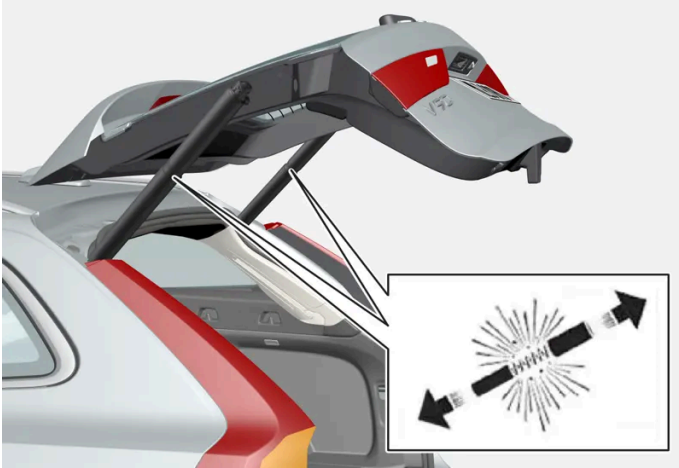
Preloaded springs for the power tailgate.
