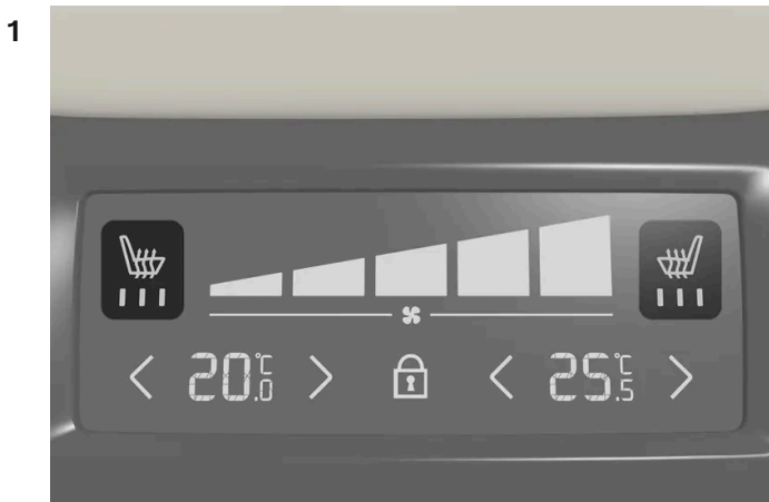
Seat heating controls and indicator lights on the rear side of the tunnel console.
