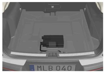
Mild hybrid vehicles have a 48 V support battery under the cargo compartment. The battery may only be handled by authorized workshop personnel.
