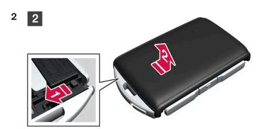
Move the catch behind the front cover to the side and slide the rear cover away from the key ring bracket.
