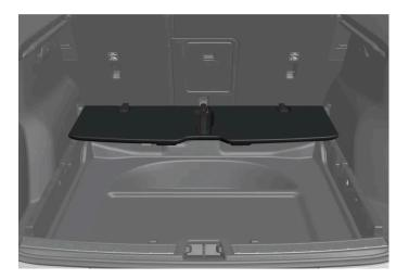
1 Lift the handle in the middle of the folding cargo compartment floor and push it forward so that it folds together.
