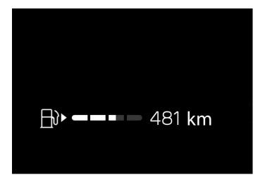
The white area in the fuel gauge indicates the amount of fuel left in the tank.
