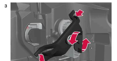
Unscrew the spring screw by turning counterclockwise, press the clips into the sides and remove the support bridge. It is simplest to leave one screw in place in the support bridge.
