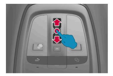
Make a steady and continuous swiping motion rearward/forward over the touch-sensitive control to fully open/close the panoramic roof. If this doesn't work, try making the motion more quickly or slowly.
