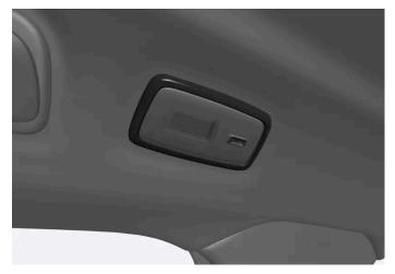
In vehicles with a panoramic roof\*, there are two lighting units on each side of the roof.
