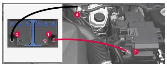
Jumper cable charging points. Engine compartment appearance may vary depending on vehicle model and equipment level.
