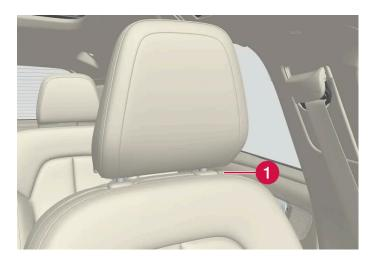
1 The head restraint can be adjusted up or down by pressing the button and manually moving the head restraint to the desired position.
