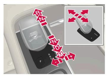
Gear selector and gear selector positions overview.
