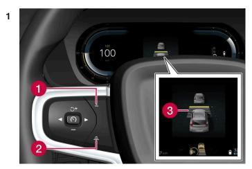
Controls for setting a time interval.
