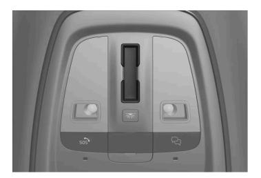
The panoramic roof and sun curtain are operated using the controls in the overhead console.
