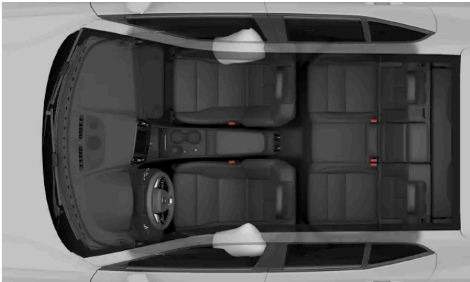
Side-collision airbags for the front occupants.
