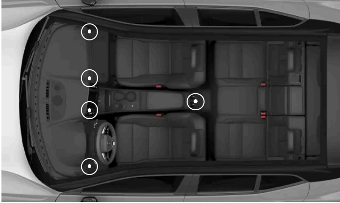
The locations of the adjustable air vents
