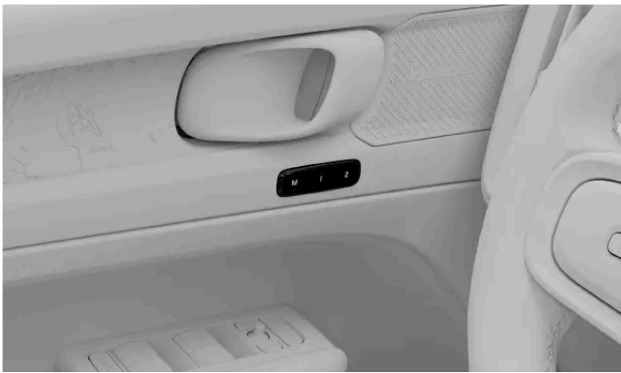
Location of the preset seat adjustment buttons
