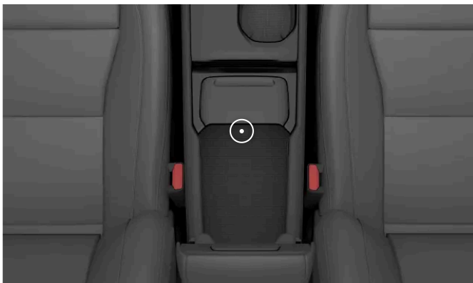
Location of the backup reader inside the center console's storage compartment.
