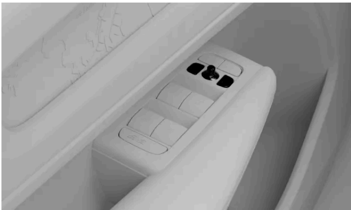
Controls for adjusting the door mirrors
