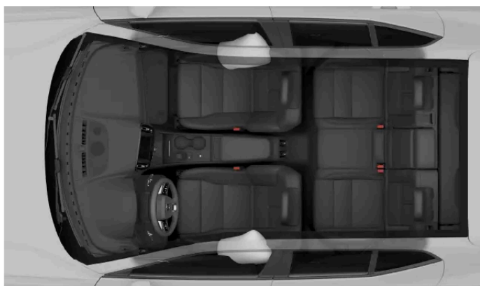
Side-collision airbags for the front occupants.
