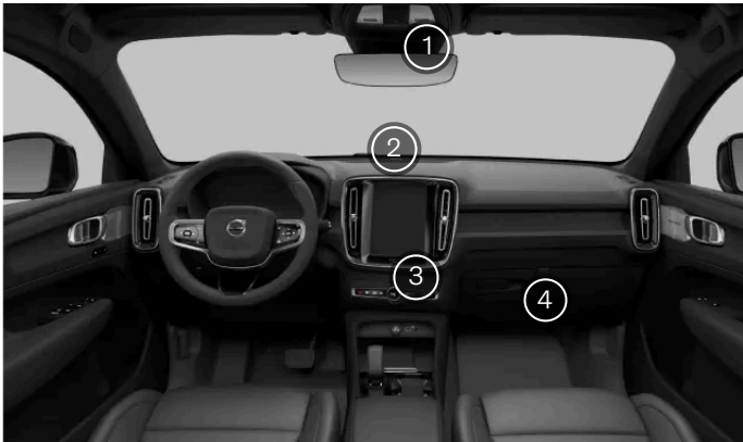
Interior climate sensors
