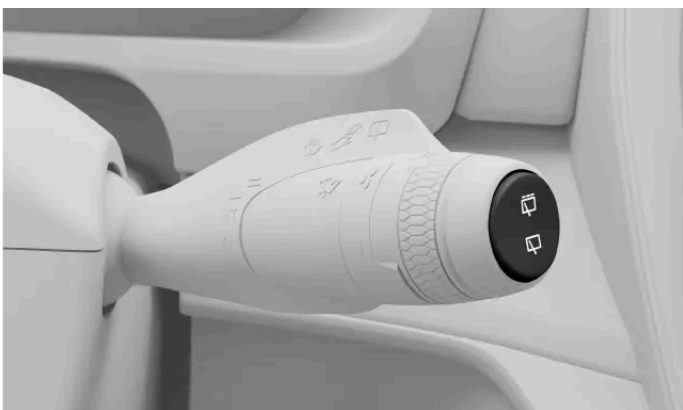
Rear wiper controls are on the right-hand steering wheel stalk.
