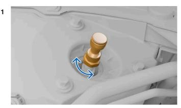
Turn the adjustment knob clockwise or counterclockwise to select a position.
