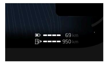
The battery meter is shown in the instrument panel at all times.
