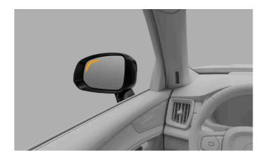
When a vehicle is detected in or approaching your blind spot, a light appears in the door mirror.
