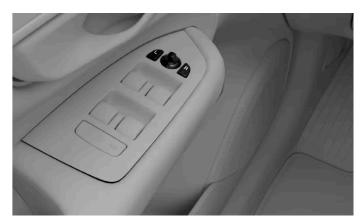
Controls for adjusting the door mirrors
