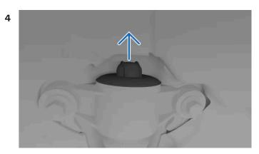
The rear wheels' suspension adjustment knob is covered by a rubber cap.
