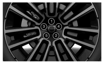
Tighten the wheel fasteners crosswise.
