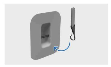
Fastening tether to top tether attachment point
