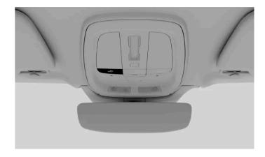
The  ${\hbox{\footnotesize SOS}}$  button is located on the roof, to the left of the overhead console.
