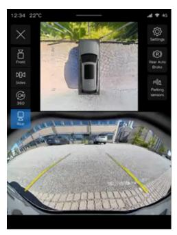
The parking view can display two views at the same time. The image shows an example of what it can look like after selecting the rear camera view, which is shown in the bottom half of the center display. The top half of the display shows an overview of your vehicle's surroundings.
