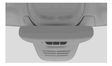
HomeLink is integrated in the rearview mirror and consists of three buttons and an indicator light. You can connect one device per button. You can add, change or delete a connection to a device.
