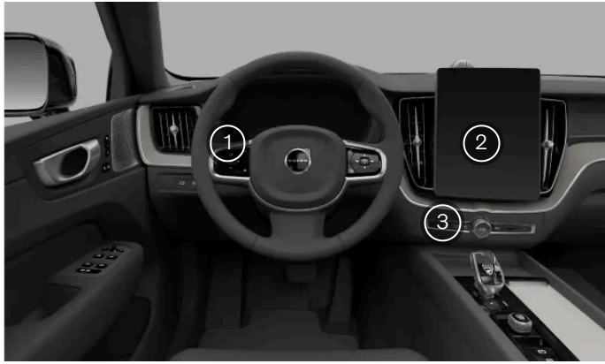
Exterior light control locations
