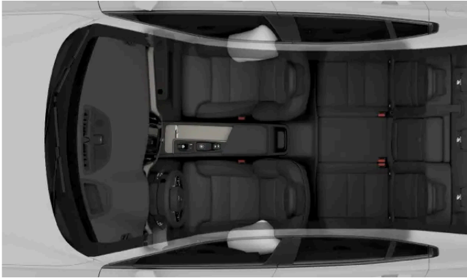
Side-collision airbags for the front occupants.
