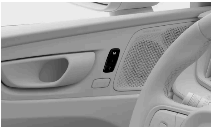
Location of the preset seat adjustment buttons
