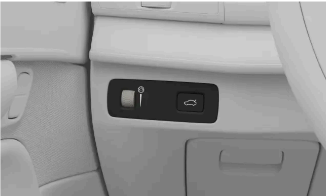
The interior lights adjustment thumbwheel
