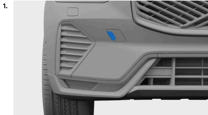
Front towing eye fastening cover
