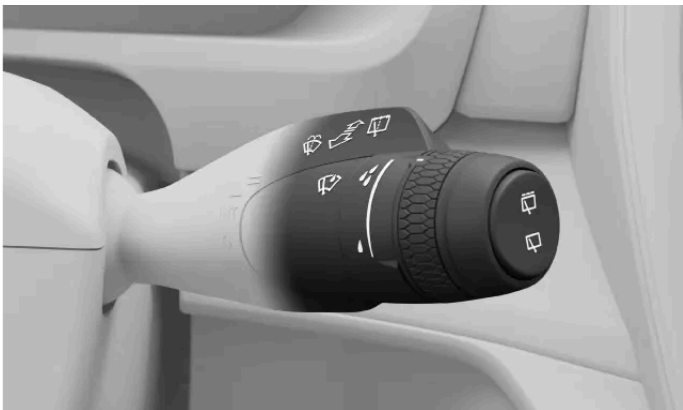
Right-hand steering wheel stalk
