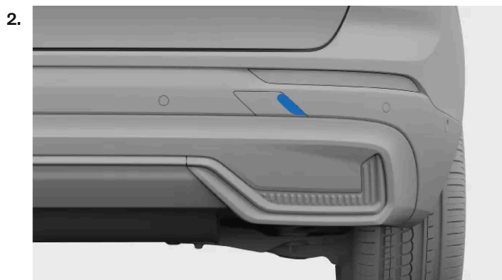
Rear towing eye fastening cover
