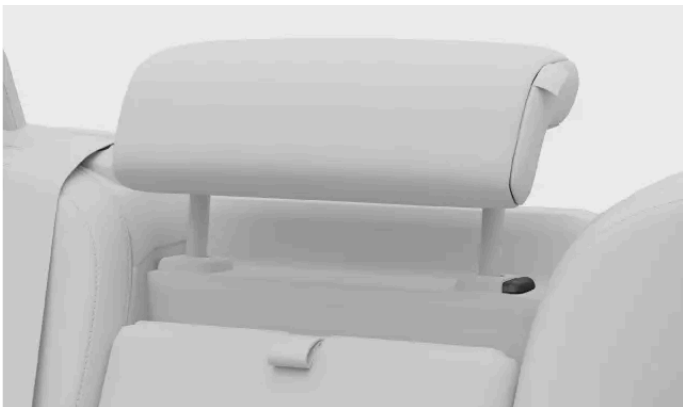
Locking button on the headrest
