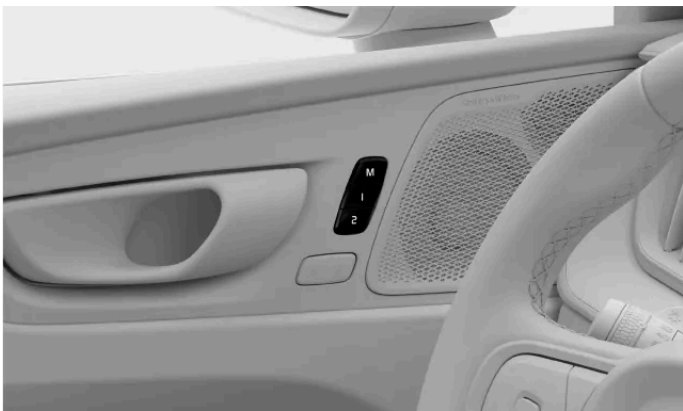
Location of the preset seat adjustment buttons
