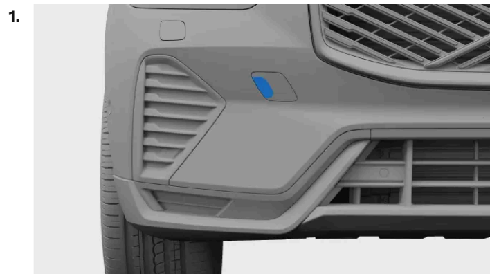
Front towing eye fastening cover
