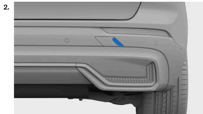
Rear towing eye fastening cover
