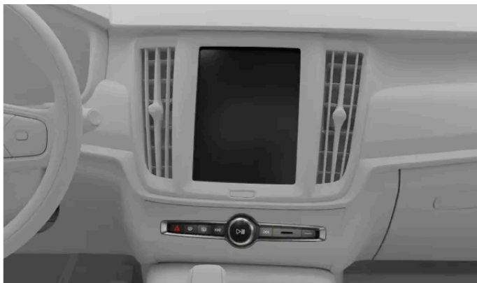
Center display and defroster buttons on the button panel below the center display
