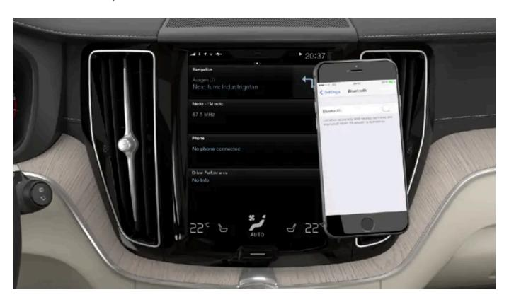
Two Bluetooth devices can be connected at the same time, but in that case, only one will be used for wireless playback. The most recently paired phone will be automatically connected to make calls, send/receive text messages, play media or use as an Internet connection <sup>[1]</sup>. It is possible to change what the phone is used for under **Bluetooth Devices** via the settings menu in the center display's Top view. The cellular phone must be equipped with Bluetooth and support tethering.
