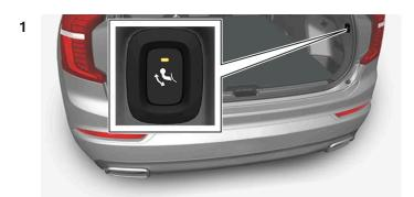
Open the tailgate. There is a button for operating the hitch on the right-hand side at the rear of the cargo compartment. Steady orange illumination from the indicator light in the button shows that the folding function is active.
