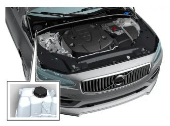
Coolant expansion tank, left-hand drive vehicle
