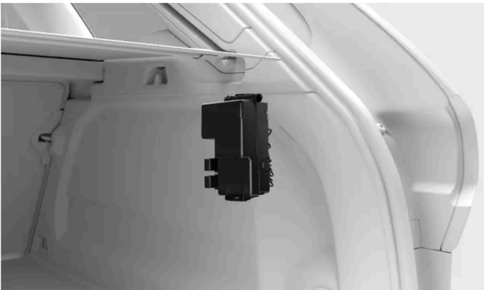
Fuse box location
