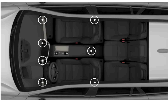
The locations of the adjustable air vents
