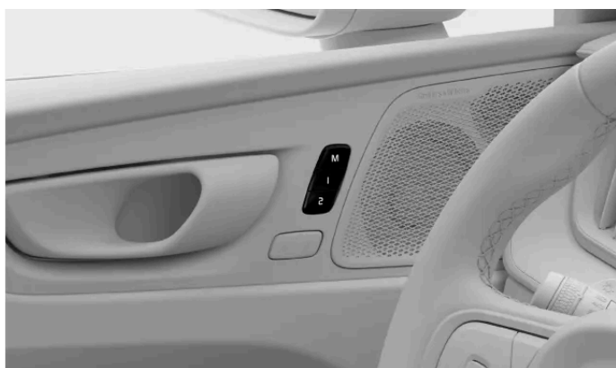
Location of the preset seat adjustment buttons
