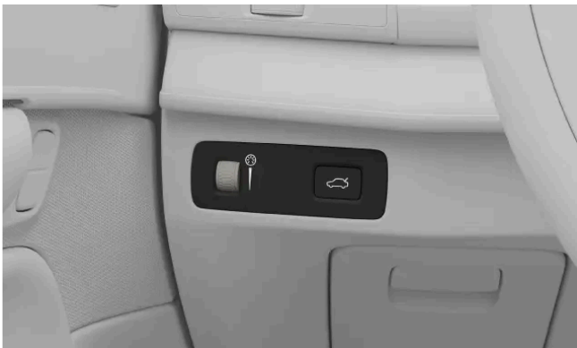
The interior lights adjustment thumbwheel
