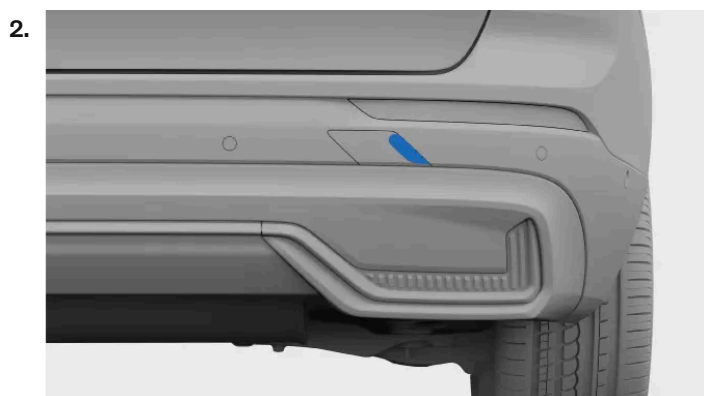
Rear towing eye fastening cover
