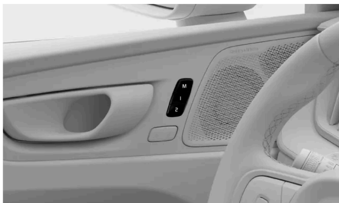
Location of the preset seat adjustment buttons
