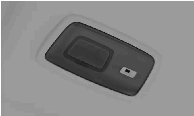
The rear seat reading lights
