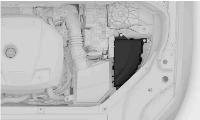
Fuse box location
