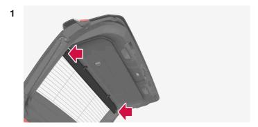
Turn the flap so that the screw side faces down and guide the pin into the bracket on one side of the tailgate.
