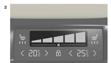
Blower controls on the rear climate panel of the tunnel console.
