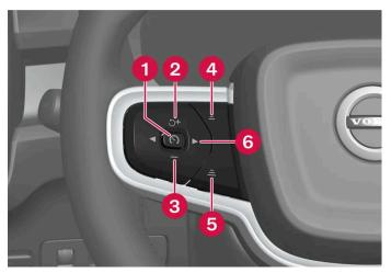
Buttons for speed-controlling functions
