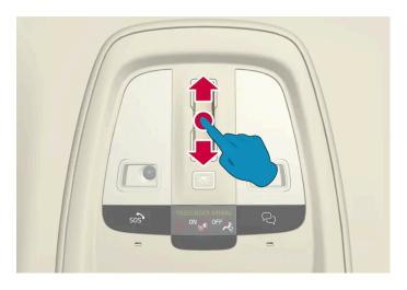
Make a steady and continuous swiping motion rearward/forward over the touch-sensitive control to fully open/close the panoramic roof. If this doesn't work, try making the motion more quickly or slowly.
