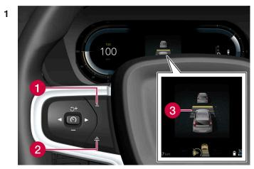
Controls for setting a time interval.
