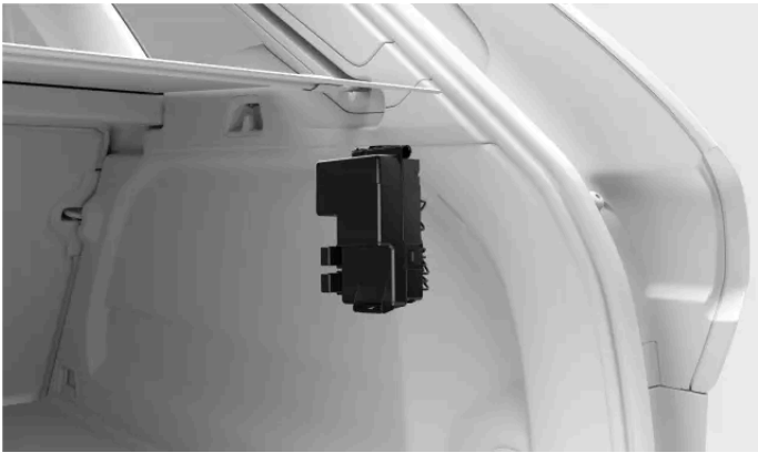
Fuse box location
