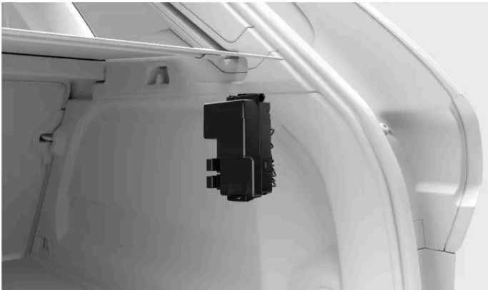
Fuse box location
