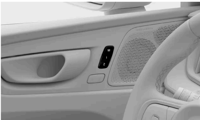
Location of the preset seat adjustment buttons
