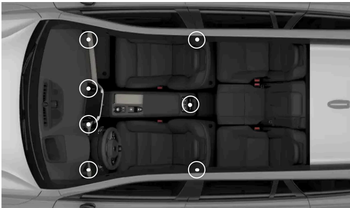
The locations of the adjustable air vents
