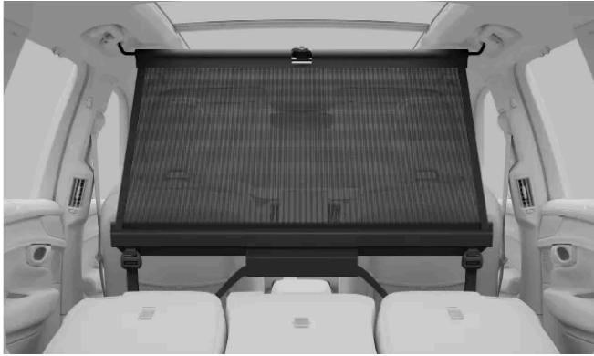
Installing behind second-row seats
