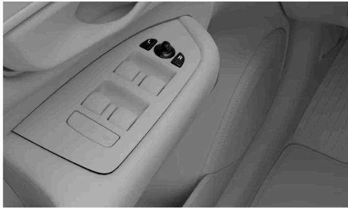
Controls for adjusting the door mirrors
