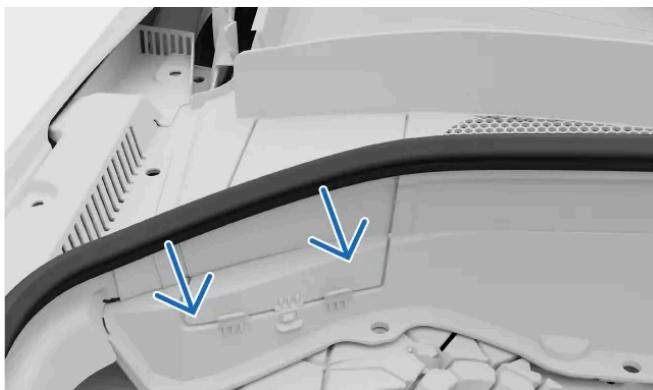
The coolant container is located in the upper-left corner of the engine compartment, underneath a panel hatch. Pull the rubber seal toward the engine compartment to access the hatch.
