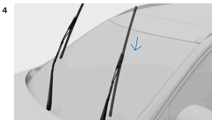
Make sure that the blade for the driver side is longer than the blade for the passenger side. Slide the wiper blade onto the wiper arm. Ensure that the pin on the wiper arm goes into the hole on the wiper blade. Push the blade into the wiper arm until you hear a click.
