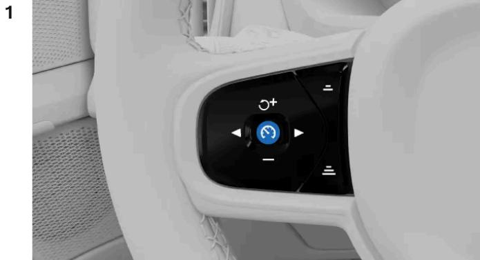
When it's safe to do so, press the Pilot Assist button
