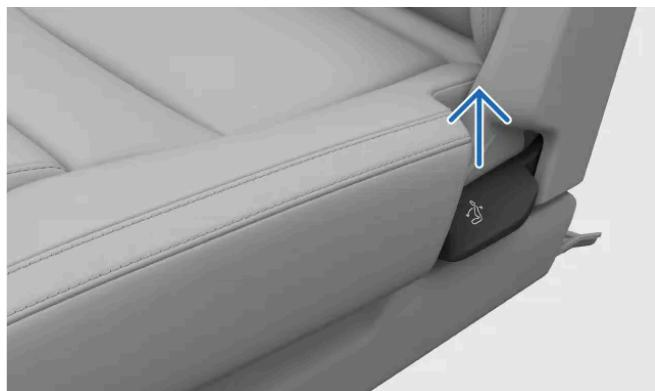
Pull and hold the handle on the side of the seat upward to unlock backrest movement.
