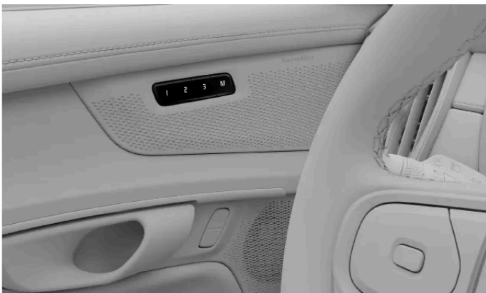
Location of the preset seat adjustment buttons
