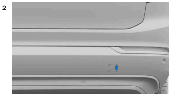
Rear towing eye fastening cover
