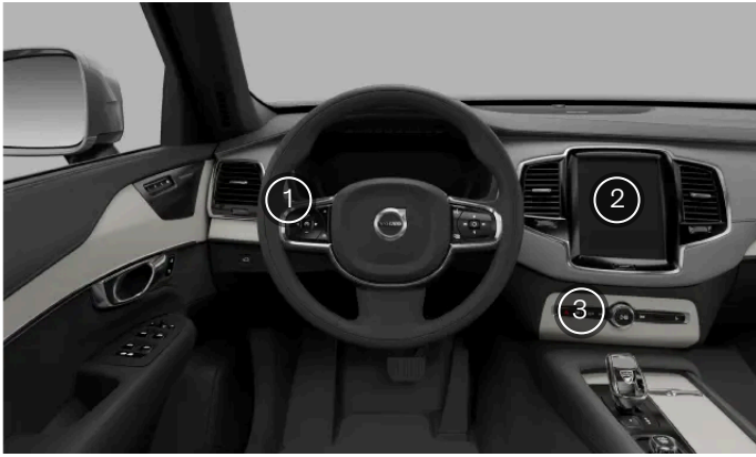
Exterior light control locations
