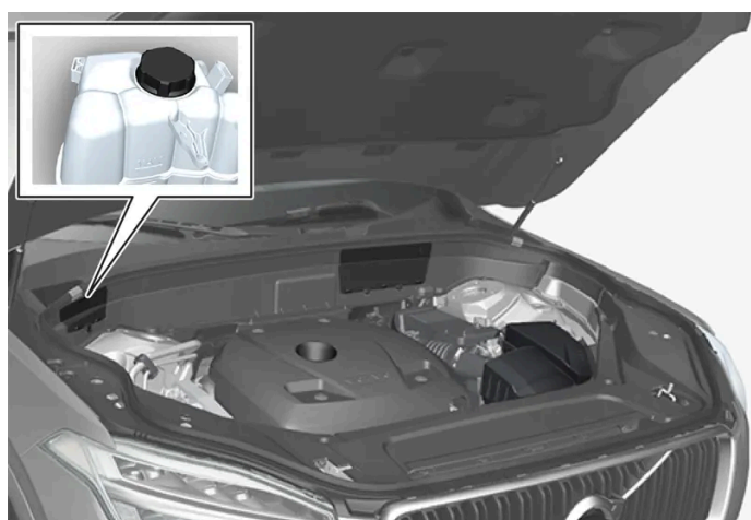
Coolant expansion tank
