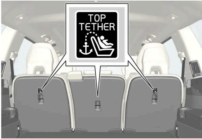
Five-seat and seven-seat models: Top tether anchors and symbols on the rear side of the second row backrests. There is no symbol for the center anchor position.
