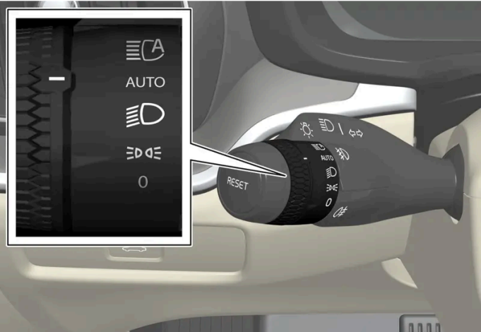
Lighting ring position.
