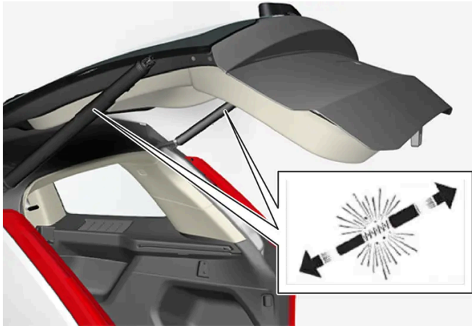
Preloaded springs for the power tailgate.
