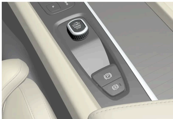
Start knob in the tunnel console.
