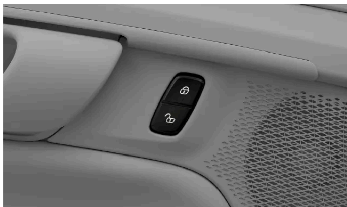
Front door button for central locking
