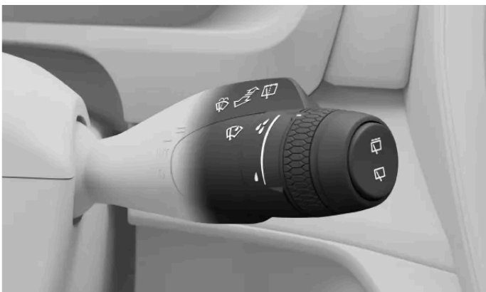
Right-hand steering wheel stalk
