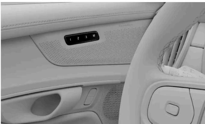
Location of the preset seat adjustment buttons
