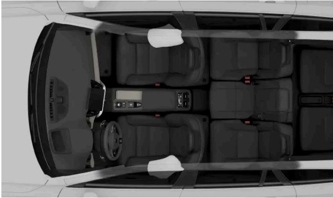
Side-collision airbags for the front occupants.
