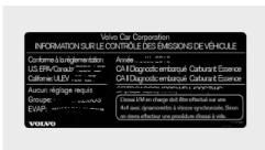
Label Vehicle Emission Control Information
