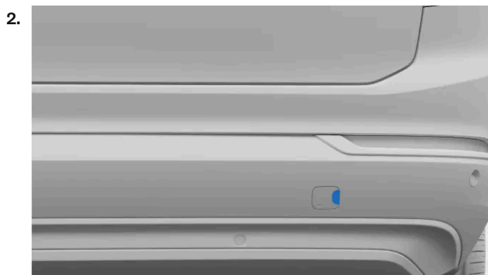
Rear towing eye fastening cover
