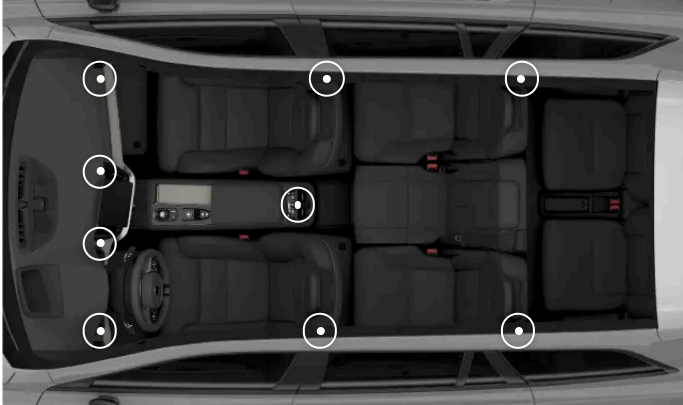
The locations of the adjustable air vents
