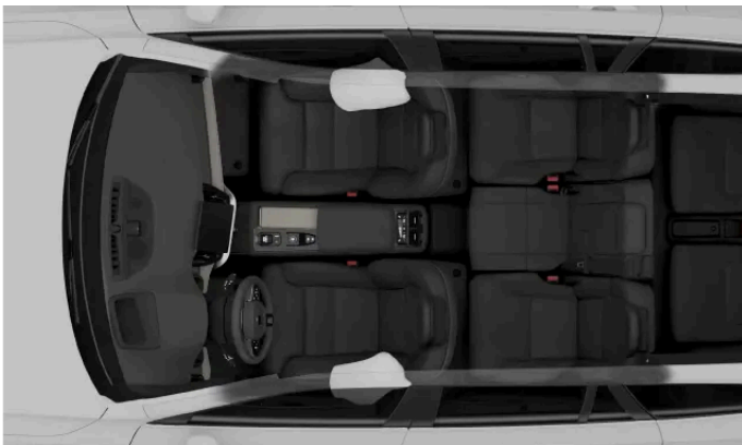
Side-collision airbags for the front occupants.
