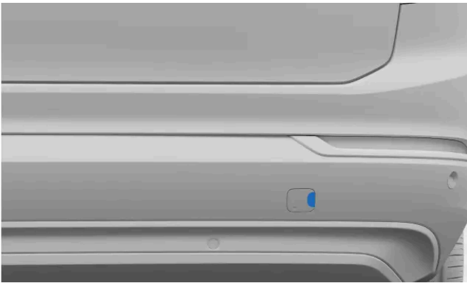
Rear towing eye fastening cover
