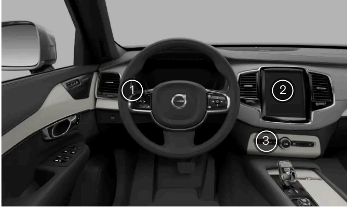
Exterior light control locations
