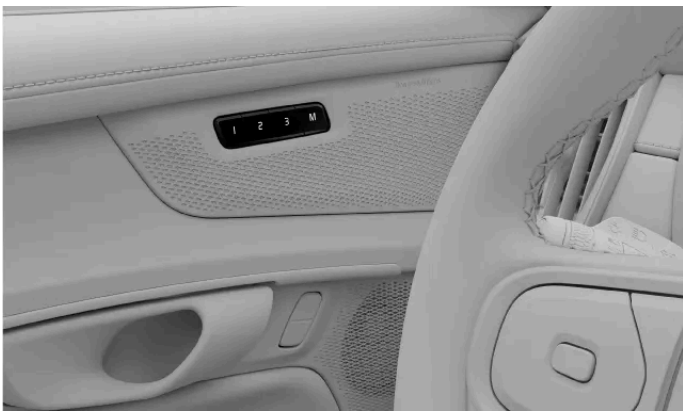
Location of the preset seat adjustment buttons
