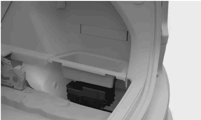
Fuse box location
