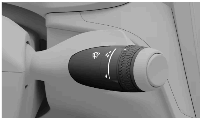
Front wiper controls are on the right-hand steering wheel stalk.
