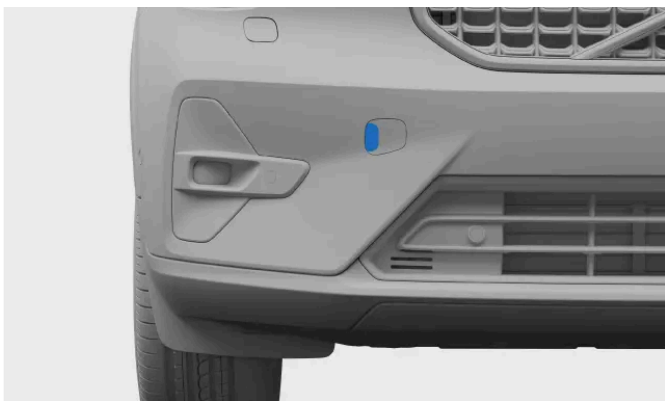
Front towing eye fastening cover
