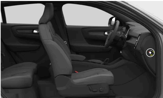
Location of the passenger airbag switch
