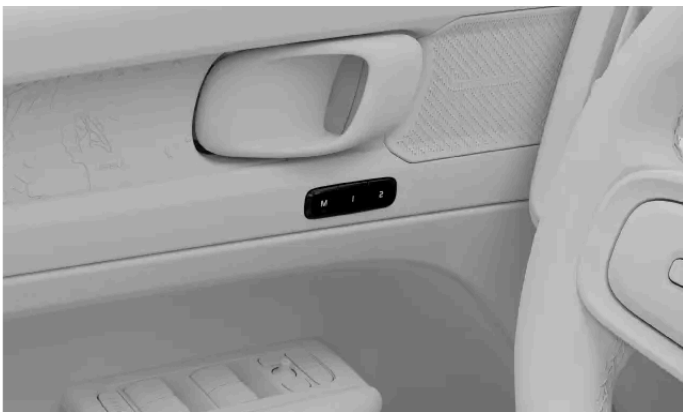
Location of the preset seat adjustment buttons
