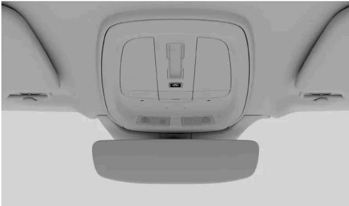
The auto lights off button in the overhead console
