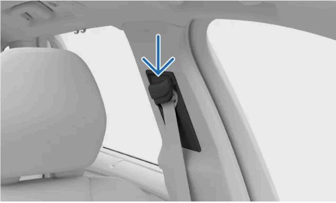
Seatbelt upper anchor point
