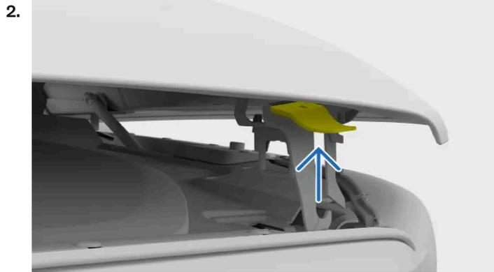
Locate the second lever on the underside of the bonnet and push it upwards.
