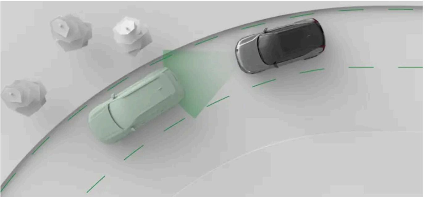
Pilot Assist actively guides your driving in a number of ways. When driving with Pilot Assist, you select the target speed. The car then manages acceleration and braking to meet that target while also adapting to surrounding traffic.
