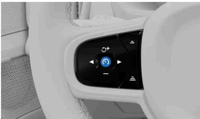
When it's safe to do so, press the Pilot Assist button
