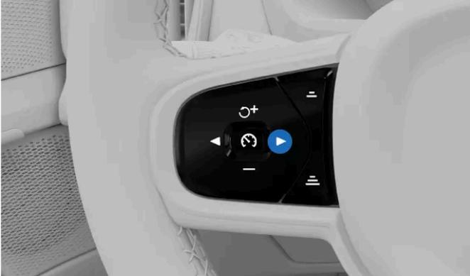
Press the switch button ► on the steering wheel.
