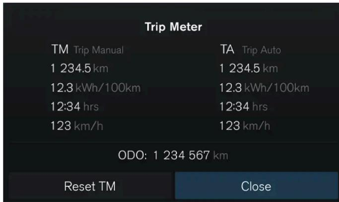
Your car has a trip meter and an odometer. The trip meter can show information on the car's driving distance and time, as well as your average driving speed.
