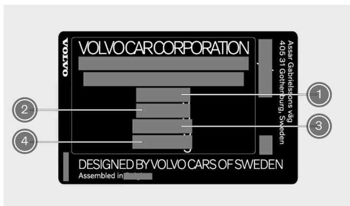
The label is located on the right-hand door pillar and will be visible when the door is opened.
