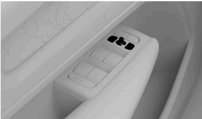
Controls for adjusting the wing mirrors
