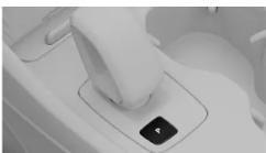
Manually engage the parking brake by pressing the parking brake button.
