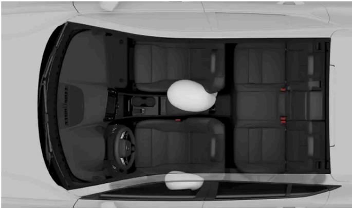
Left-side collision airbags for the front occupants. In a right-side collision they deploy on the other side of each front seat, mirrored compared to the depicted scenario.
