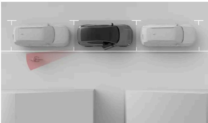
Door opening alerts are designed to warn you of passing traffic so that you don't open a door in its path. These alerts can be provided when the car is stationary or moving very slowly<sup>[1]</sup>.
