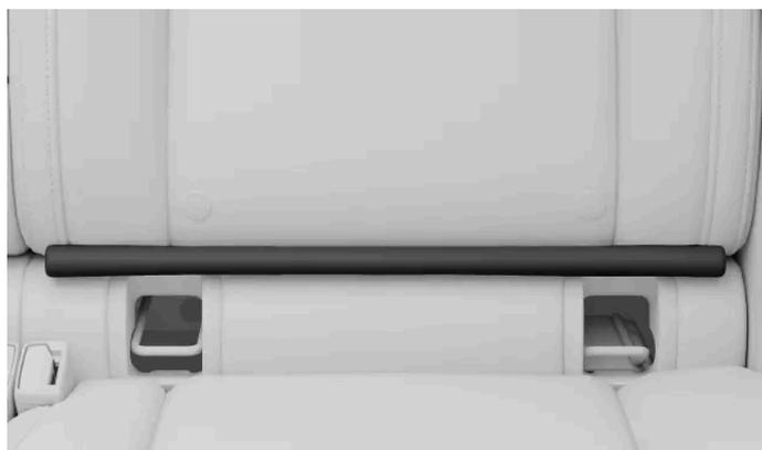
The folded ISOFIX flap, tucked into the gap above the anchorage points
