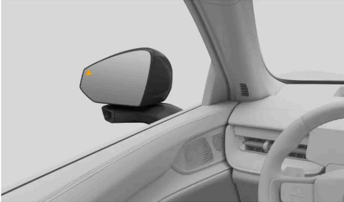
When the car detects traffic that is about to pass close to the car's sides, a light appears in the wing mirror. If you begin to open the door on the side of the detected traffic, the alert intensifies. A sound alert can occur along with the visual alerts depending on how urgent the warning is.
