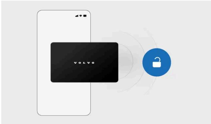
Once you've set up a digital key on your device, it works in the same way as your other keys. If your device has UWB<sup>[1]</sup> capability, your car will be able to detect the digital key from a distance. If your device doesn't have UWB capability, the digital key works as a key card.
