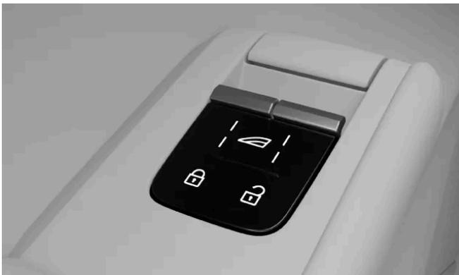
Press the window symbol
