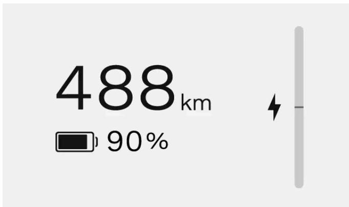
Your range is primarily related to your car's battery level and your driving practices but external conditions can also be a factor. The battery level and expected range are displayed in the driver display. The expected range is calculated based on your driving pattern, both current and historical.
