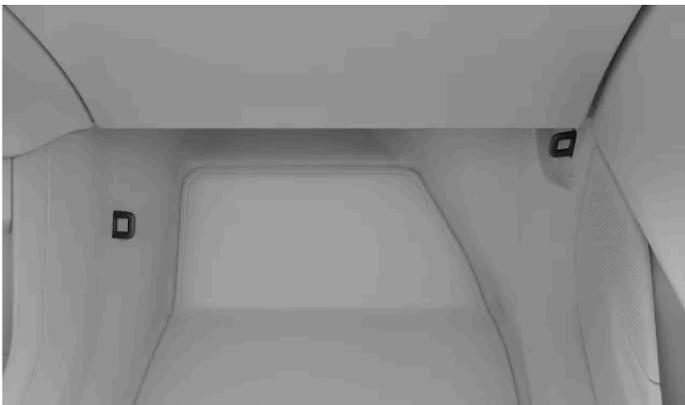
With the front lower tether accessory<sup>[1]</sup>, the anchorage points for the front passenger seat are located on the sides of the seat's footwell.
